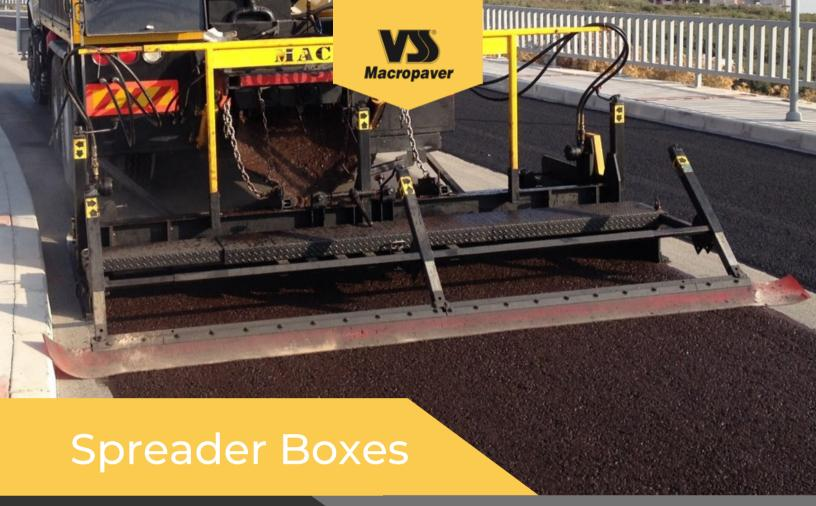
Slurry & Micro Surfacing Boxes
